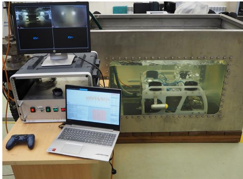
Fig. 2. External view of the manufactured "Model of the device for laser underwater cleaning of the surface of objects from biofouling"
