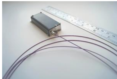
Fig. 1. External view of the laser diode module LMD-50.
